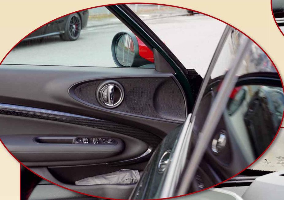
The 10 cm bass-midrange drivers of the Match system are installed in the doors
